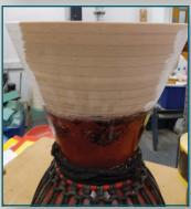
Our DT Technician, Dave Harding, a super talented carpenter, took this job on board. He spent quite a few hours on the laith shaping MDF to the correct shape and size. He then was able to level off the damaged drum and attach the new component to the drum base.
